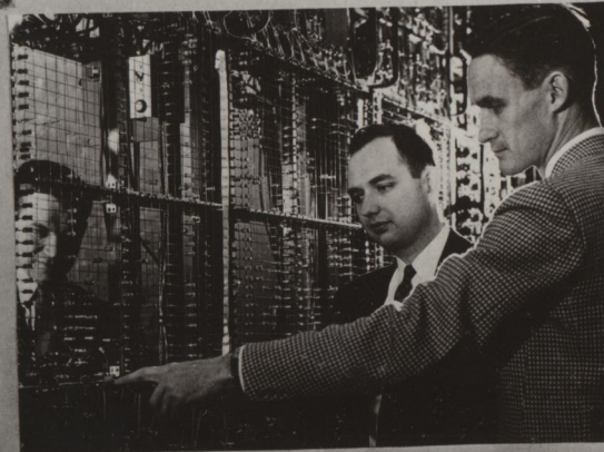
CONTROL The control element of WHIRLWIND I selects the operation to be performed by energizing the appropriate one of the 32 horizontal lines shown in the photograph. The selected line then opens the appropriate channels to allow operation pulses to pass to other parts of the computer.
